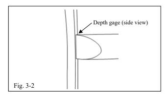
Align the adjustment tool to the edge of the door, with the angle edge positioned toward the inside of the door (Fig. 3-2).
