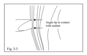
**Sealant Issue:** To push back sealant; align the adjustment tool to the edge of the door, with the angle edge positioned toward the inside of the door (Fig. 3-3).
