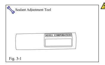
NOTE: Use the adjustment tool to verify if sealant is close to the door's edge. This must be done prior to **Door Edge Guard** installation to allow for proper fit (Fig. 3-1).
